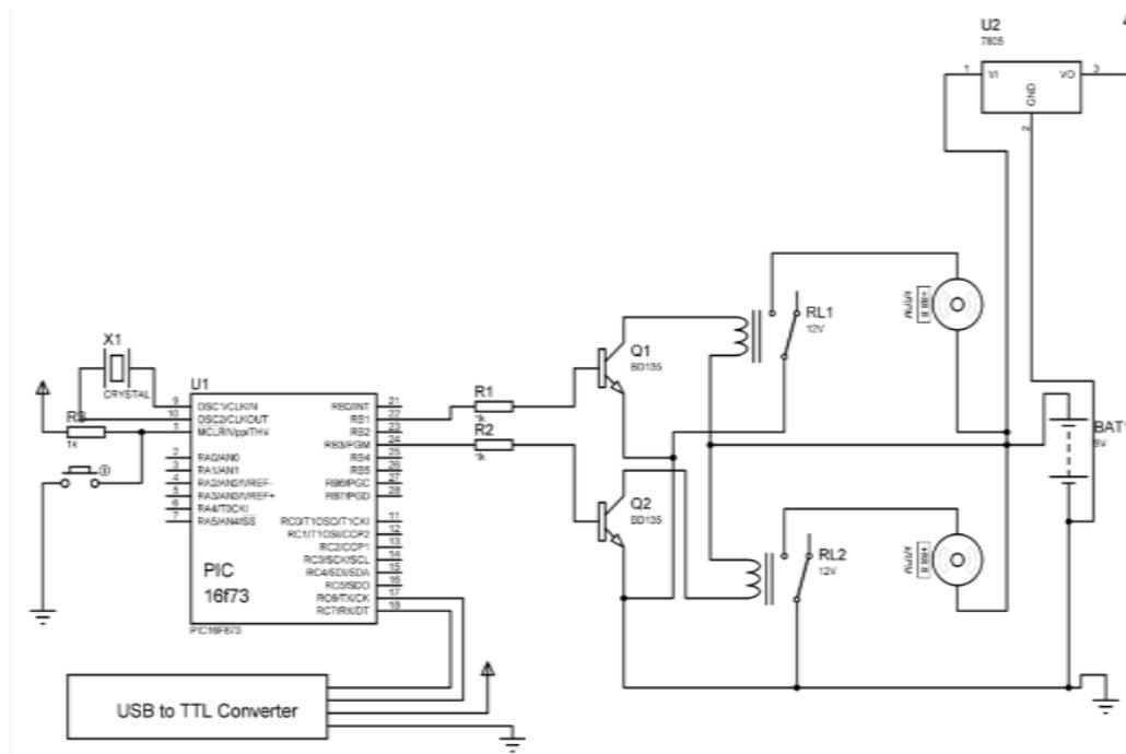
Fig.8: Implemented interfacing circuit diagram.
