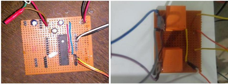
Fig.9(a) Main or Brain circuit and (b) Relay or motor control circuit
