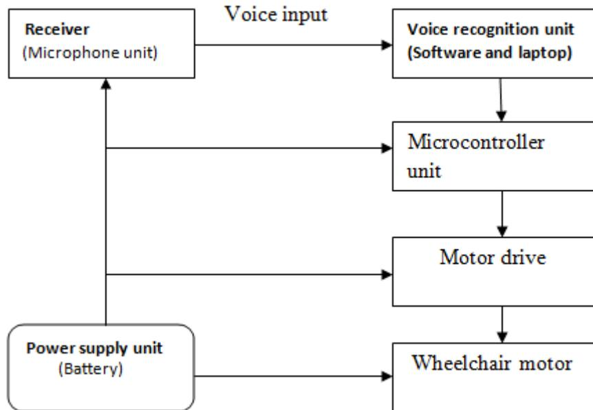
Fig.5: Wheelchair control system block diagram.
