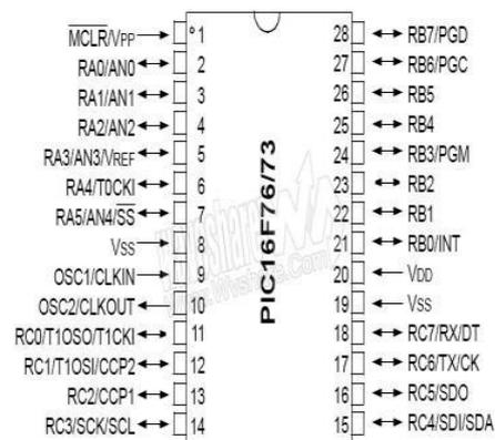
Fig.4 PIC 16F73 microcontroller pin diagram.
