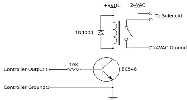
Fig.3(a) Relay Circuit
