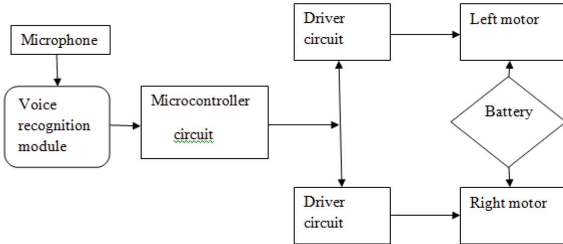
Fig.7: Basic Components of Wheelchair
