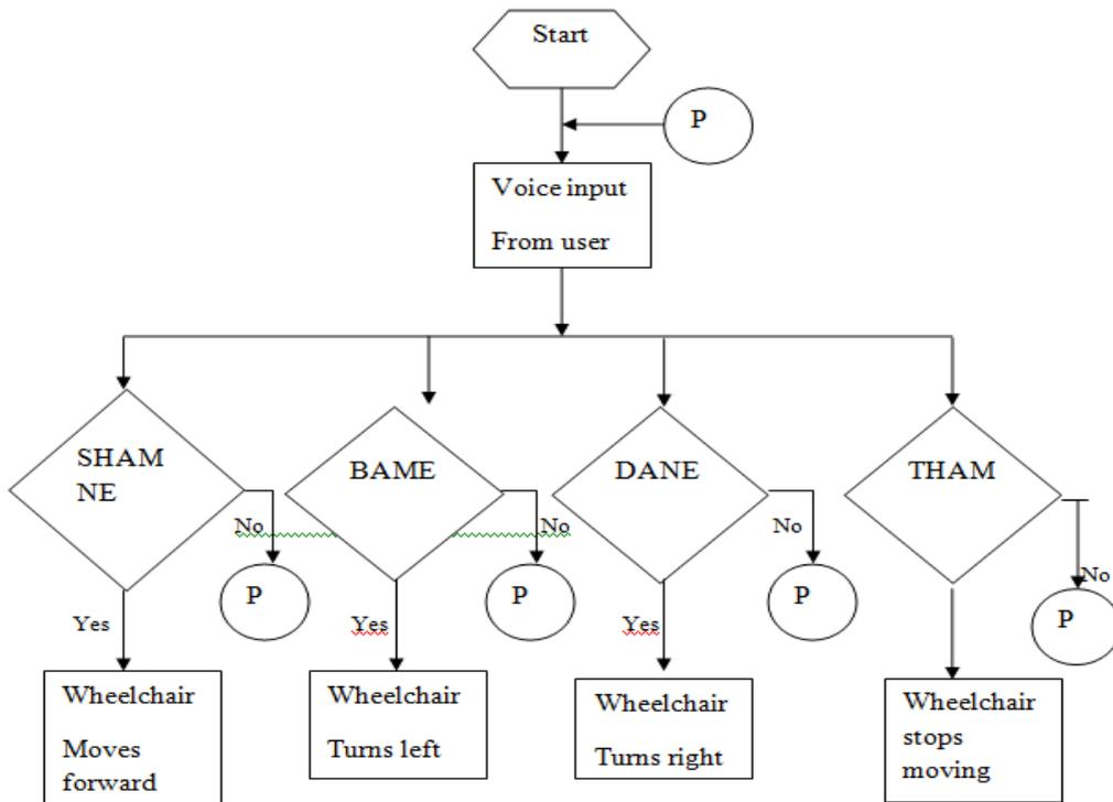
Fig.11: Voice controlled motion of the wheelchair.
