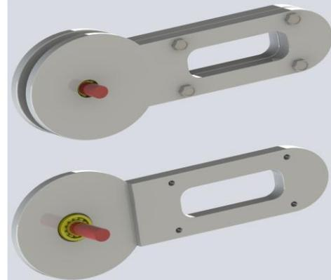
Fig. 4: 3D model of waist-hip connector
