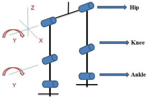
Fig. 1: The gait model of mechanism
