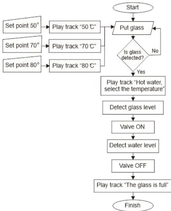
Fig. 6 Hot water system
