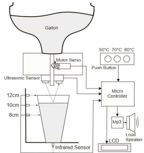
Fig. 4 The automatic water dispenser system
