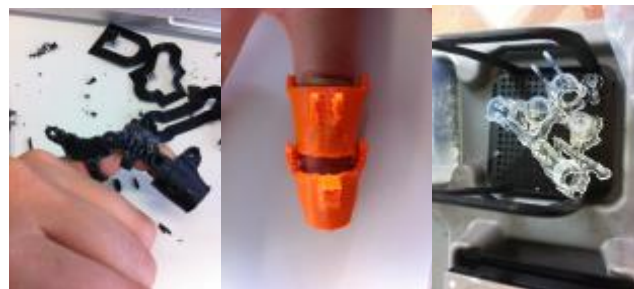
Figure 12. Printed Process whit PLA material, 13. Innoflex Flexible material, 14. Clear resin 3D printed material.
