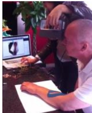
Figure 11. 3D Scanning Process forearm and back of the hand. https://youtu.be/7QCgrAymrIM
