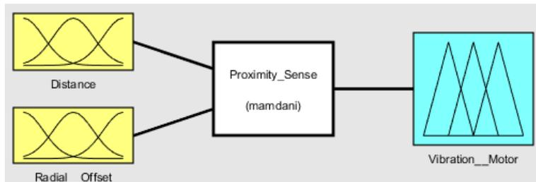
Fig. 3. Inputs and Outputs for fuzzy logic model
