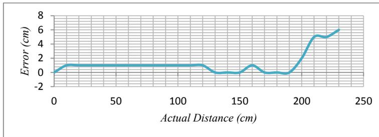
Fig. 2. Error relation with distance for ultrasonic sensor
