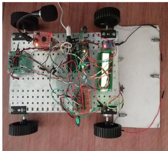
Figure 4, Hardware setup of the smart wheelchair
